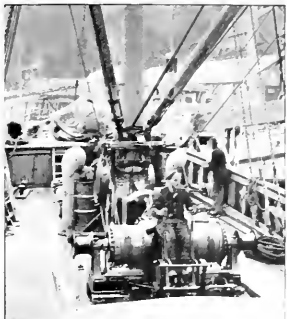
A silent hoist "AA" double drum winch driven by 60 horsepower gas engine in action on board the motorship Teco of the British Columbia Cement Company, Vancouver, B. C.
